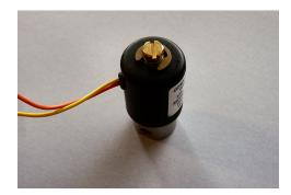
2. Remove the sealing screw from the top of the solenoid:
