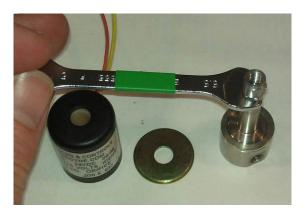
6. View of the disassembled solenoid valve:
