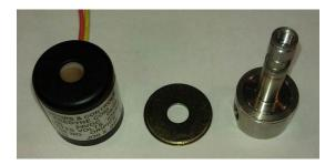
5. Unscrew the central pillar of the valve using a 5.5 mm spanner, and disassemble, taking care not to lose any parts:
