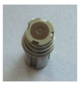
8. Check the lower body of the valve for any particles and blow out with compressed air:
