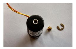
4. Remove the coil assembly and stepped washer noting orientation:
